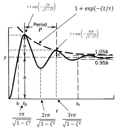
– Decay ratio (DR): a function of damping coefficient only!
