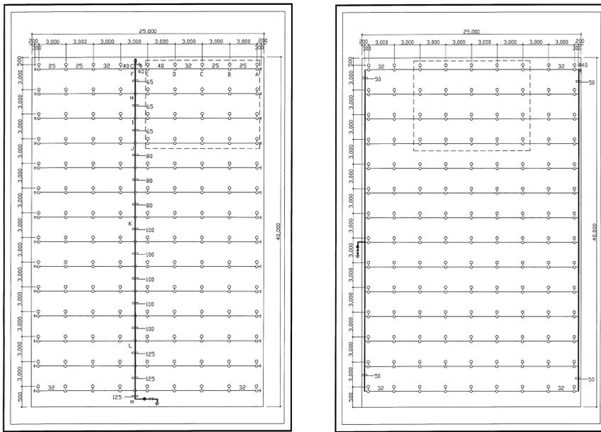
Fig. 1. Plan View of 1000m<sup>2</sup> Tree and Grid System Case
