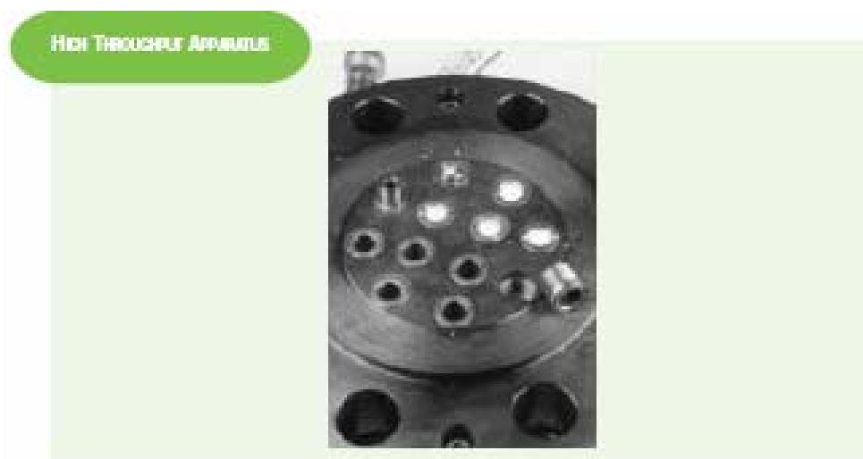
High throughput screening apparatus rapidly tests activity and selectivity of heterogeneous catalysts.
