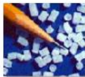
Diameter 3 mm Length 5-15mm Hardness 2-3 Mohs CO 2 Content 99.95%
