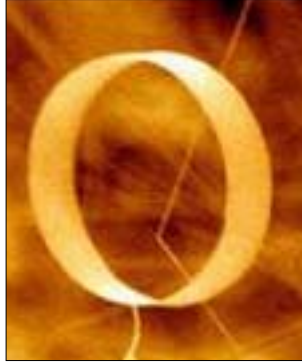
그림 8. Zinc oxide nanostructure synthesized by a vapor-solid process. (Image courtesy of Prof. Zhong Lin Wang, Georgia Tech))
