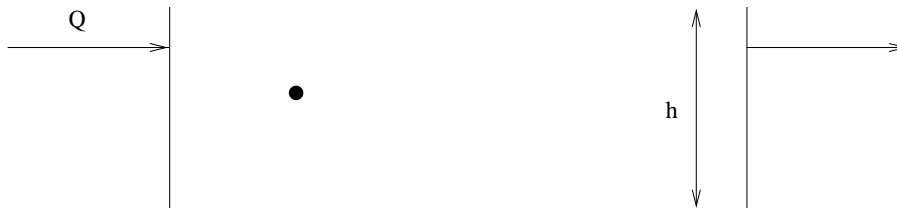
Figure 3: Settling in an ideal settling basin. The basin depth is h , the surface area is A .
