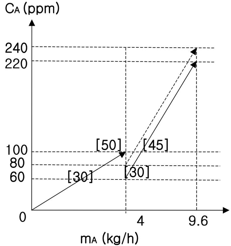
Limiting water profiles after inlet concentration shift
