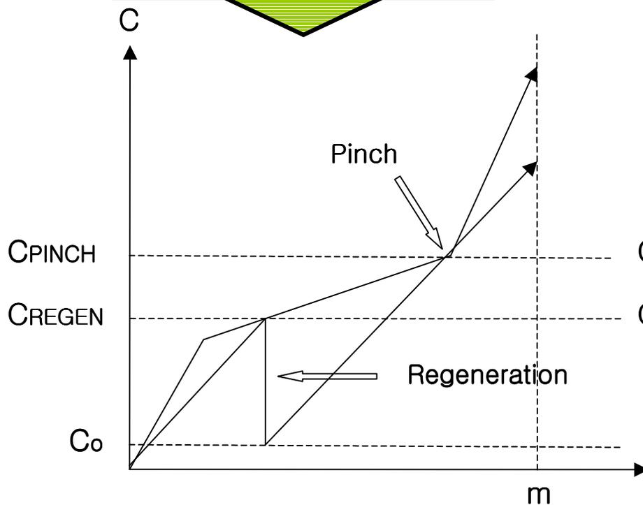
Regeneration of water reduces the flowrate of freshwater and wastewater
