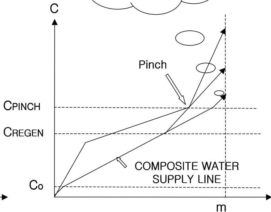
Composite water supply line indicates that the water flowrate is not minimised
