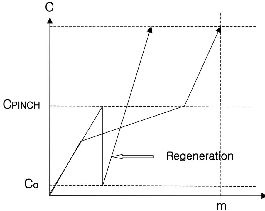
Minimum flowrate set by slope of limiting composite curve below  $C_0$
