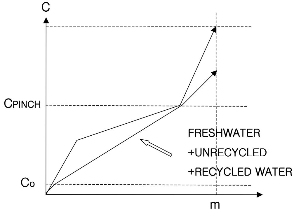
A Composite of the water supply before and after regeneration
