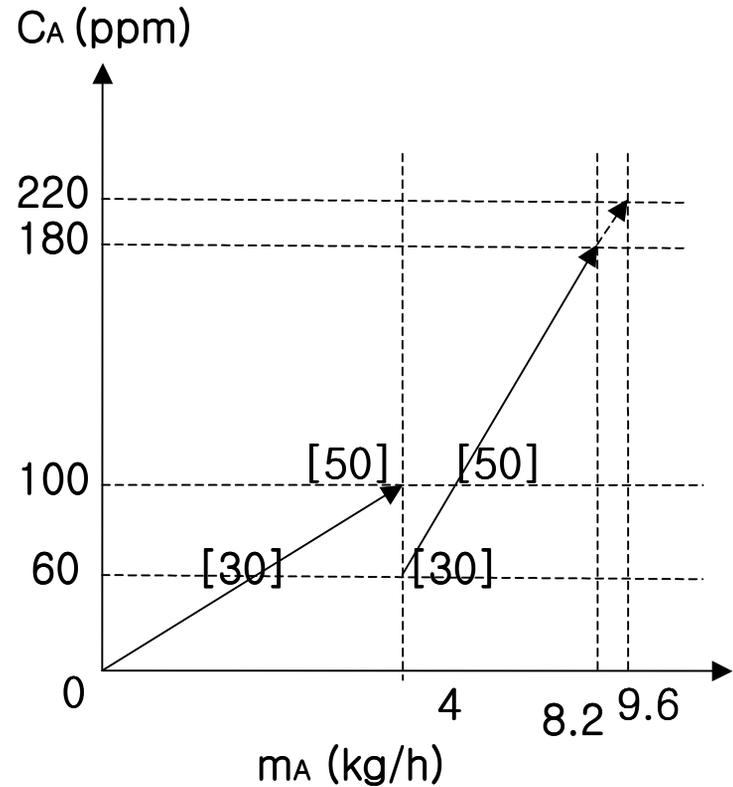
Limiting water profiles after inlet and outlet concentration shift
