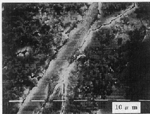
Fig. 6. Microstructure of SiC/SiC composite after thermal shock test.
