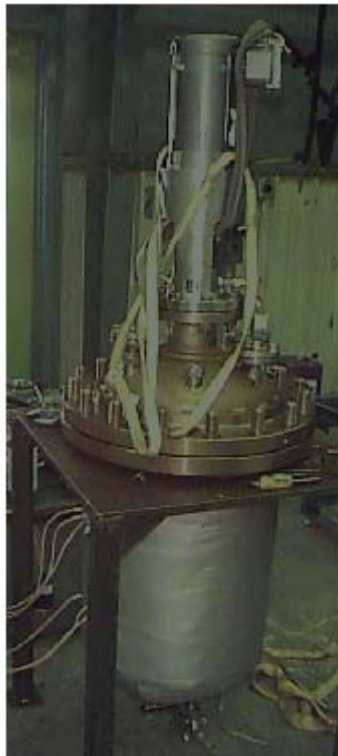
Figure 2. One of five, 2-m tall, 75-liter hydrolysis (or oxidation) vessels at LLNL's pilot-scale waste treatment facility. Rapid hydrolysis of mixed-waste chloro-solvents to produce water-soluble products was demonstrated here and in same scale laboratory systems (Figure 4).
