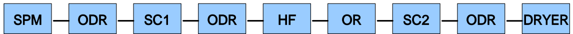
Fig. 4. Typical RCA cleaning process flow, with overflow rinse(OR) or overflow dump rinse(ODR) steps between each chemical treatment.
