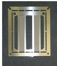
Individual Reactor shim plate 1 of 5 types that are diffusion bonded
