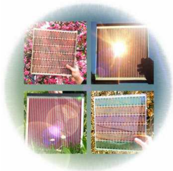
Figure 1. Gratzel Cells - Solar Cells Based on Titanium Dioxide (Gratzel cells are named after their inventor, the Swiss scientist Michael Gratzel. Instead of silicon, they rely on titanium dioxide ( \text{TiO}_2 ) - a cheap and widely available material used in everything from paints to coffee whiteners.)- referece: http://sites.google.com/site/pakilinks/gratzel-solar-cell
