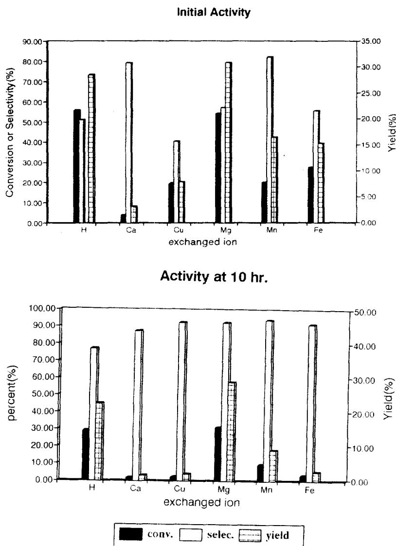
Fig. 1. Initial Activity and Activity at 10 hr. of various Ion Exchanged ZSM - 22.
