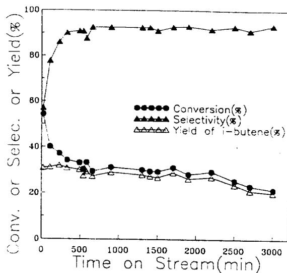
Fig. 2. Influence of Time on Stream on Conversion , Selectivity and Isobutene Yield over Mg - ZSM - 22.
