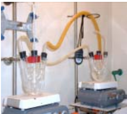
Fig. 1. The reactor for titanium dioxide -alumina mixture.
