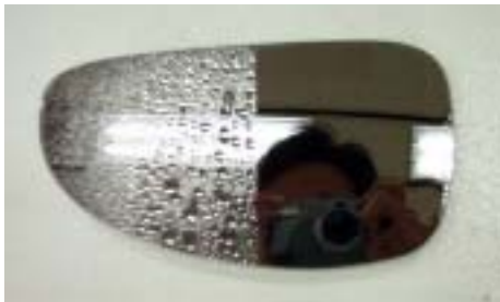
Fig. 3. Effect of photocatalyst coating on car side mirror
