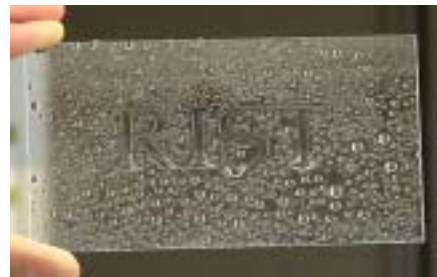
Fig. 4. Photocatalyst coating on acryl surface
