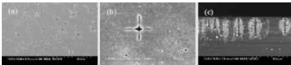
Fig. 2. FE-SEM image of anodizing the Si wafer
