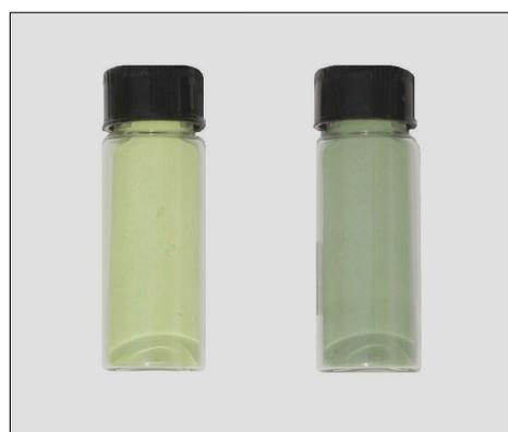
Fig. 4. The color of tungsten samples after 10 hours at  $650^\circ C$  under the helium condition.
