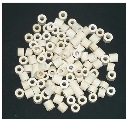
Fig. 3. Raschig-ring formed K/MgO catalyst
