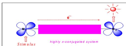
Figure 1. Scheme of organometallic compound as molecular wire.
