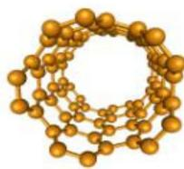
*Double-walled carbon nanotube*
