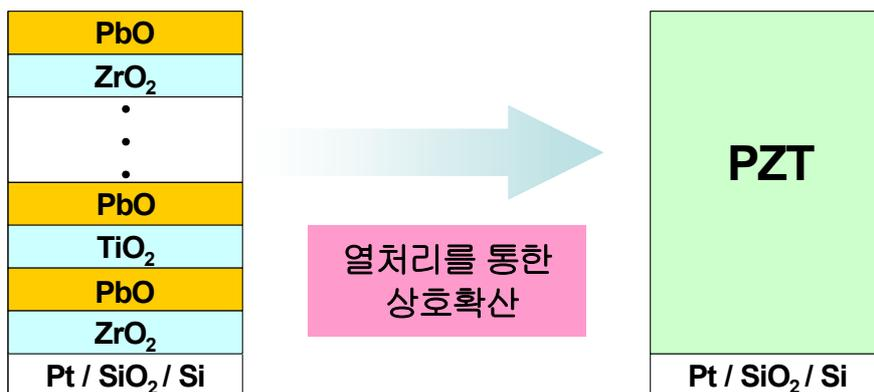
Fig.2 Schematic diagram of PZT thin film preparation.
