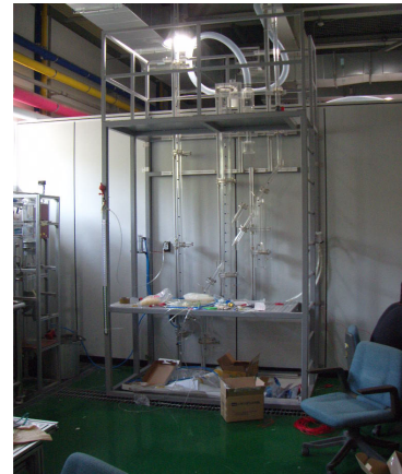
Fig. 2. 1in-ID cold-bed circulating Fluidized Bed.
