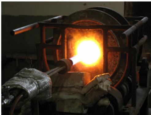
Figure 1. High temperature rotary slag test apparatus
