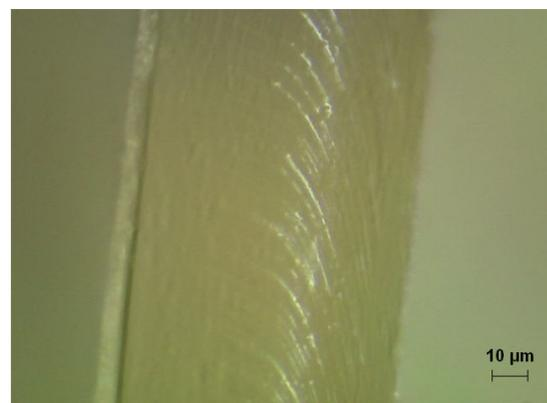
Figure 4. Photograph of TEOS coating of quartz crystal resonators.
