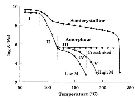
I : glassy (below  $T_g$ ) II : leather-like (at  $T_g$ ) III : rubber-like (rubber plateau) IV, V : sliding motions of molecules
