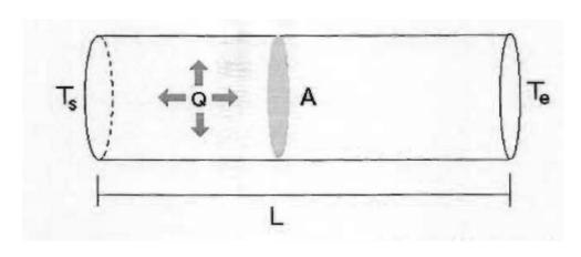
$$\begin{split} \frac{d}{dx} \left( k \frac{dT}{dx} \right) + Q &= 0 \,; \qquad 0 \leq x \leq 1 \\ k &= 3.3 \text{ J/°Cms} \,, \\ Q &= 10 \text{ J/sm} \,, \\ T|_{x=0} &= 1 \,, \\ q|_{x=1} &= 1.25 \text{ J/m}^2 \text{s} \,. \end{split}$$
