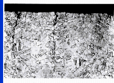
Transgranular SCC of brass
