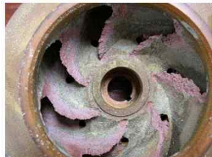
Solid erosion corrosion of impellers in slurry media
