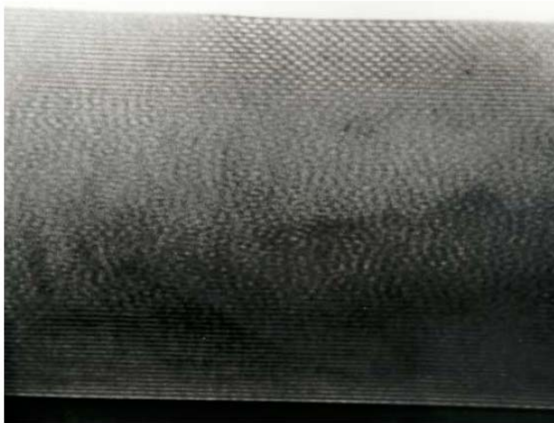
TEM cross-section through 500 nm mesoporous silica (surfactant: F127)
