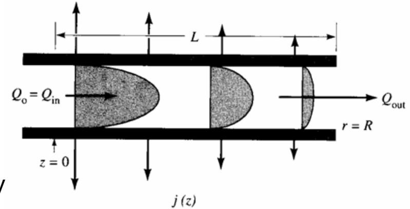
$$u_r = -\frac{1}{r} \int_0^r r \frac{\partial u_z}{\partial z} dr \quad u_r = -RU_o f'(z) \left[ \left( \frac{r}{R} \right)^1 - \frac{1}{2} \left( \frac{r}{R} \right)^3 \right] \quad u_r(R, z) \equiv u_R(z) = -\frac{RU_o}{2} f'$$
