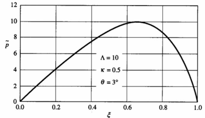
Max. pressure increases with increasing viscosity, speed, bearing length; why?
