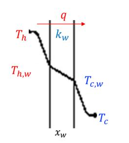
$$\delta q = \frac{\Delta T_i}{R_i} \rightarrow \begin{pmatrix} \Delta T_i = T_h - T_{h,w} \\ R_i = 1/(h_i dA_i) \end{pmatrix}$$
