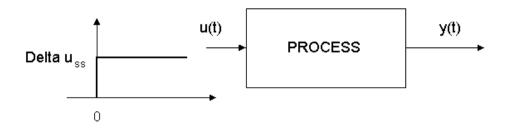
Not all but many SISO(single-input single-output) chemical processes show step responses which can be well approximated by that of the **First-Order Plus Dead Time(FOPDT)** process.
