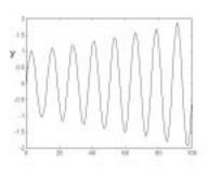
step 4 Calculate and implement PID parameters using the the Ziegler-Nichols
