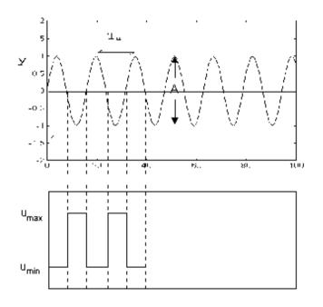
$$K_u = \frac{4(u_{max} - u_{min})}{\pi A}, \quad T_u: \text{ from the repsonse}$$
