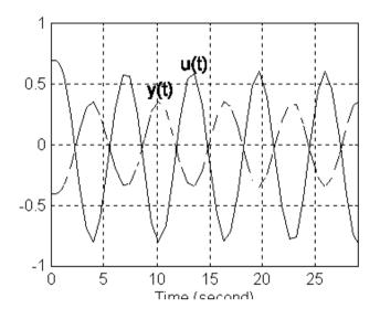
•  $K_u$  is the largest  $K_c$  for closed-loop stability under P-control. When  $K_c = 0.5K_u$  under P-control, the closed-loop approximately shows 1/4 (Quarter) decay ratio response. This roughly gives 50% overshoot.
