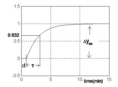
The FOPDT process is represented by three parameters
