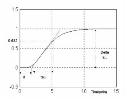
• Drawing a tangent is apt to include significant error, especially when the measurement is noisy. To avoid this trouble, the following method is recommended:
