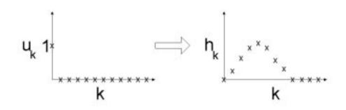
Finite Impulse Response (FIR) Model: Model for which there exists N such that
